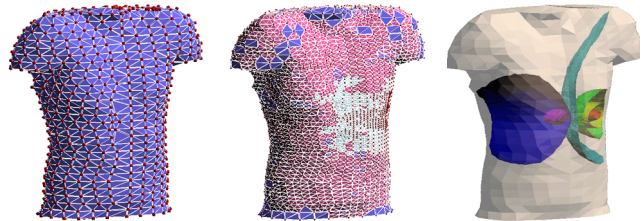
Figure 16: ECG field analysis example. On the left the initial grid; on the right the quasi-hierarchically refined grid (four levels). Red balls indicate active basis functions, cells of different colors indicate the support of basis function on different levels. Initial surface grid courtesy of the Center for Scientific Computing and Imaging, University of Utah.
